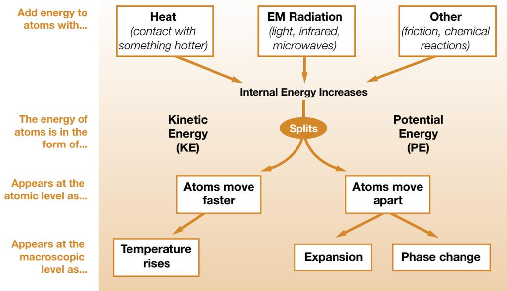
**Atoms and Energy Can Help.** Thinking atomically helps connect added energy (top row) to observed changes (bottom row). All the ways of adding energy shown increase the internal energy. This increase is split between increases in kinetic and potential energy. The former is seen at the atomic level as faster atoms and at the macroscopic level as increased temperature. Increases in potential energy involve moving atoms farther apart, which can cause expansion and phase change.
